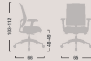
LV12 – LV22 Poltrona ergonomica con braccioli regolabili e oscillante mov. 19. Ergonomic armchair with adjustable armrests and oscillation mov. 19.
